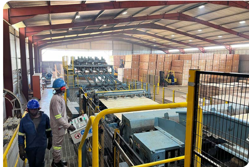
A veneer plant in Mozambique. Veneers are thin sheets of wood of uniform obtained by sawing, slicing or peeling (rotary cutting).
